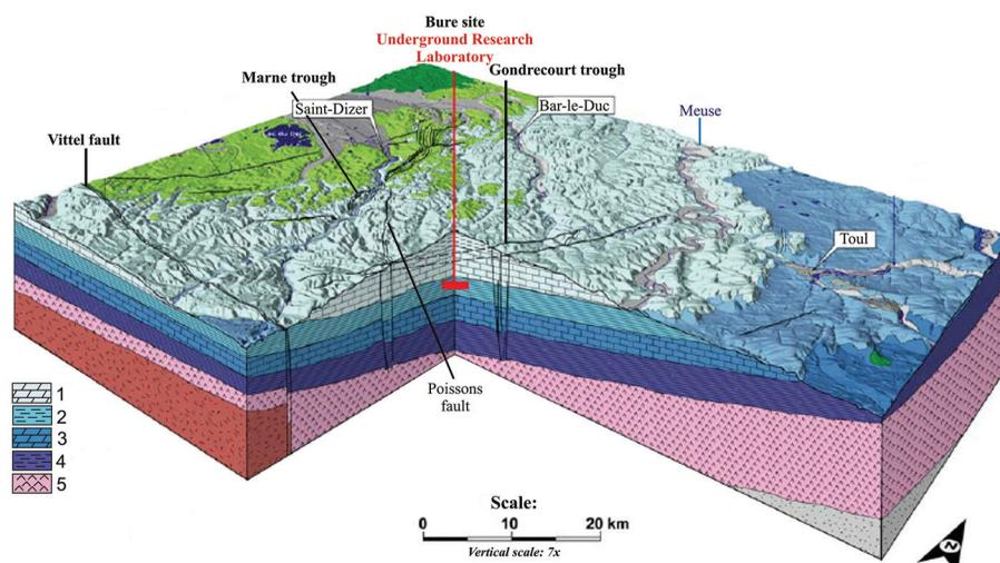
**Fig. 3.** 3D block diagram of the geological structure of the Meuse/Haute-Marne sector (after ANDRA, 2005b). 1 – Oxfordian (micritic and ooidal limestones); 2 – Callovian–Oxfordian (clays); 3 – Middle Jurassic (ooidal and bioclastic limestones and calcareous polyliers); 4 – Lower Jurassic (clays); 5 – Triassic (sandstones and evaporites).
