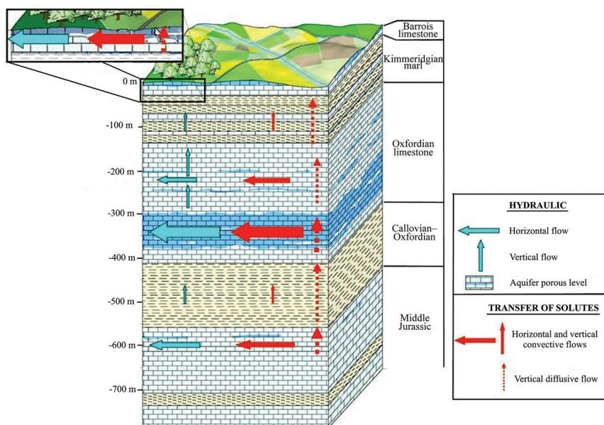
**Fig. 4.** Schematic representation of water flow and solute transport in the geological medium in its initial state at the Bure site (after ANDRA, 2005b).
